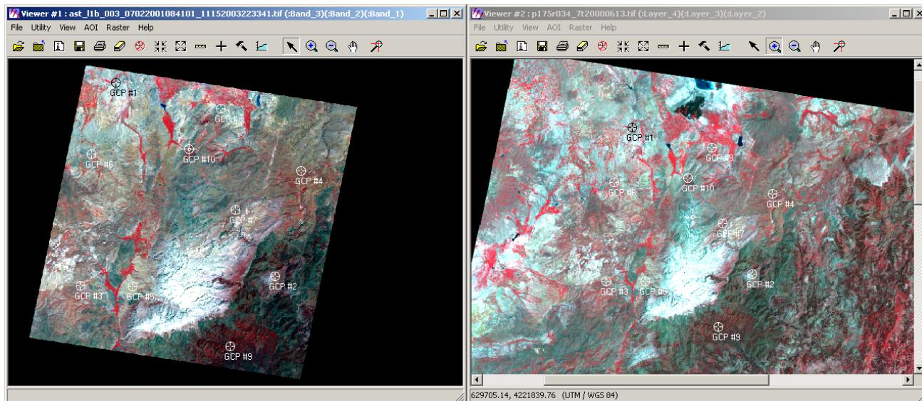
10. Note the Root Mean Square (RMS) error for each point in the GCP Tool menu to examine the accuracy of each GCP match. A good goal is to have a total RMS error of less than half a pixel (15 for a Landsat image).
