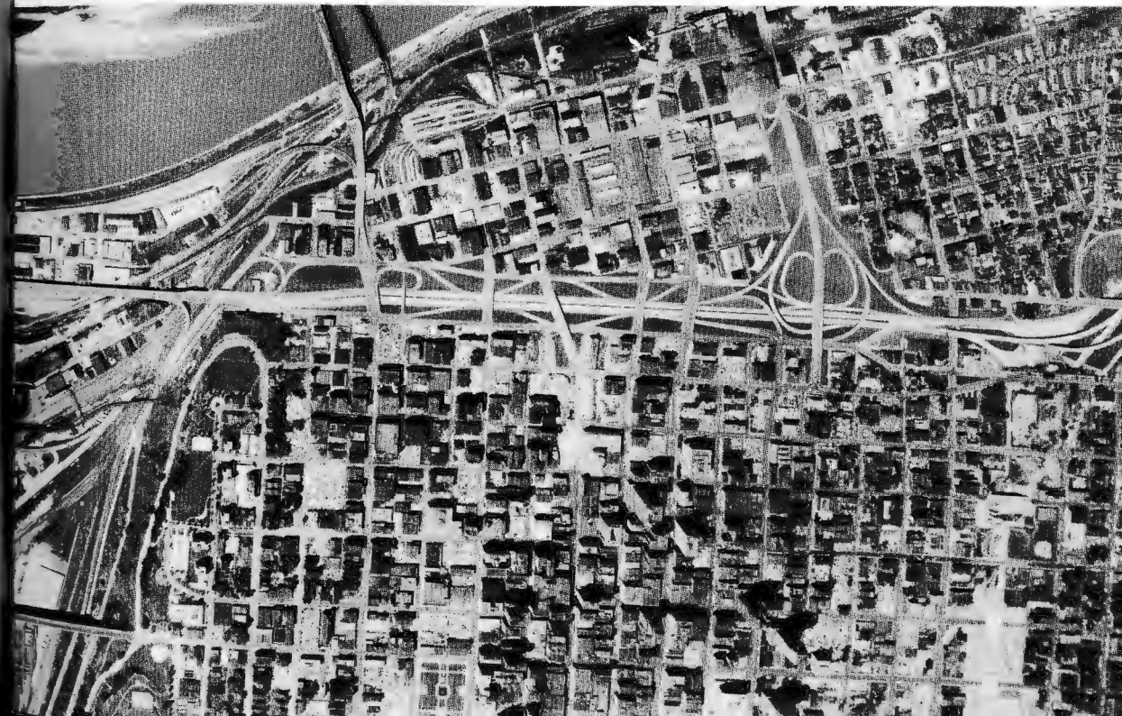
30. Spotting a break in street patterns at Kansas City, between old Missouri River-oriented grid and later gridiron to the south, highway planners chose this confusion zone as a location for Interstate 70—U.S. 24/40 east-west. Thus, highways and urban renewal have wiped out many breaks.
